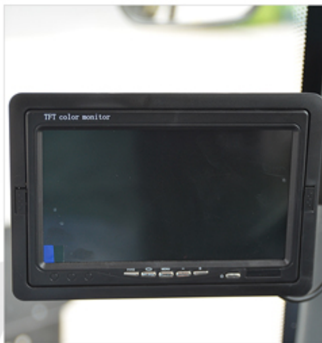
Rear view video system. Includes a rear view camera and a 7-inch monitor in the operator's cab
