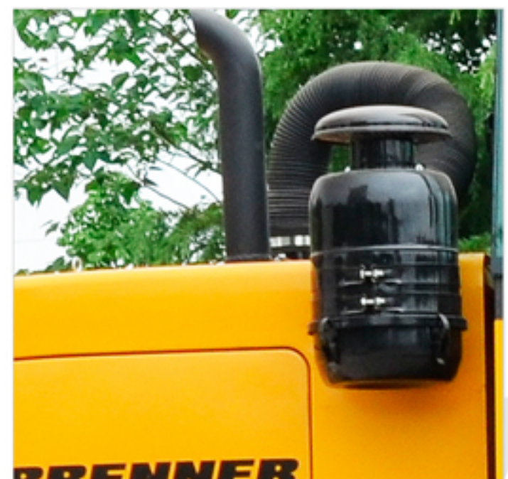
Additional air filter in oil bath
