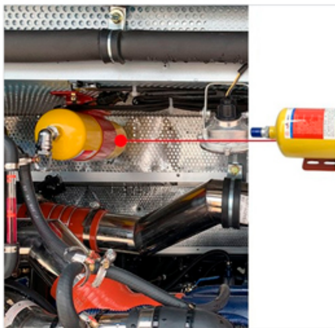
Automatic fire extinguishing system for the engine compartment with an additional button in the operator's cab
