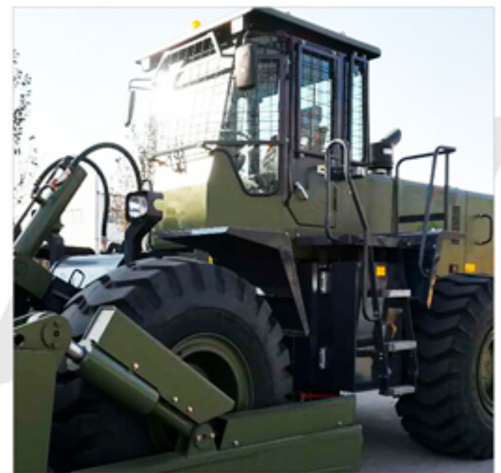
Protective grilles on the cab windows
